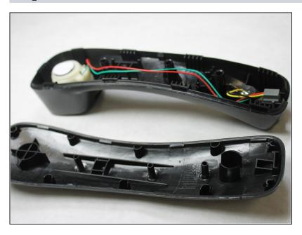
After separating the two sections of the handset, it should look as shown.
