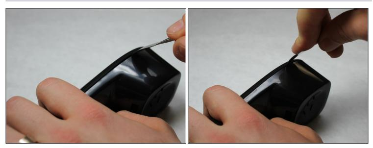
Separate the two sections of the handset by pushing them apart with the tip of the metal spudger or opening tool.
