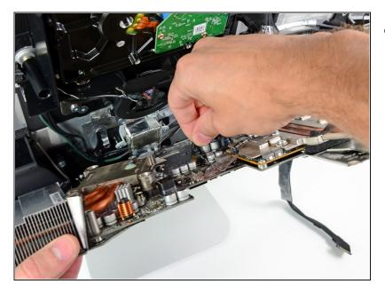
Disconnect the LCD temperature cable by pulling its connector up and out of its socket on the logic board.
