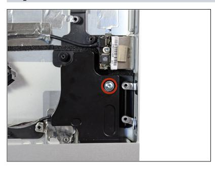
Remove the single 13 mm T10 Torx screw securing the right speaker to the outer case.
