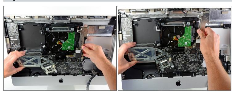
• Slightly pull the logic board away from the back of the outer case, then lift it upward to clear the lower front face of the outer case.
