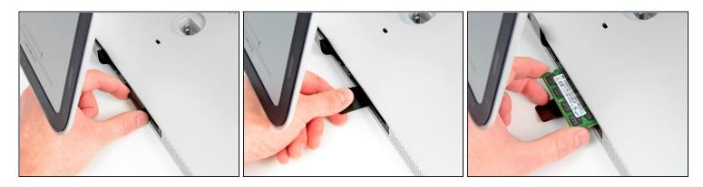
• Repeat the process in the previous steps to remove the RAM module(s) from the other side of the RAM bay.
