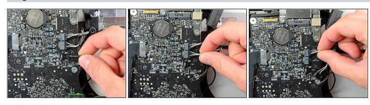
• Disconnect the microphone, left speaker, and right speaker cables by pulling their connectors toward the right side of the iMac.
