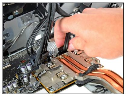
Being careful not to damage the socket on the logic board, gently pull the hard drive SATA data cable straight out of its socket on the logic board.
