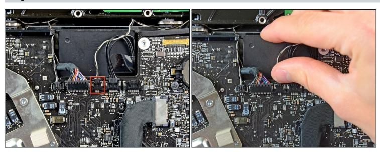
• Pull the optical drive thermal sensor connector straight up from its socket on the logic board. Pull parallel to the board.
