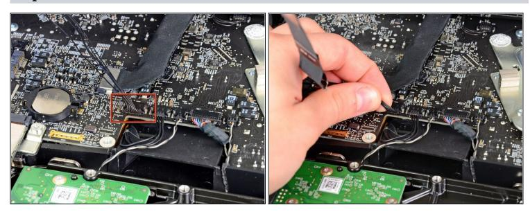
• Disconnect the LCD thermal sensor cable connector from its socket on the logic board.
