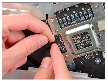
Pull the CPU fan/ambient temperature sensor connector toward the bottom left edge of the iMac and out of its socket on the logic board.
