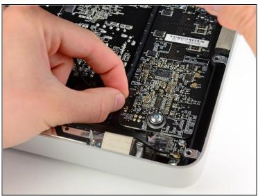
• Pull the vertical sync cable connector out of its socket on the LED driver board near the top left corner of your iMac.
