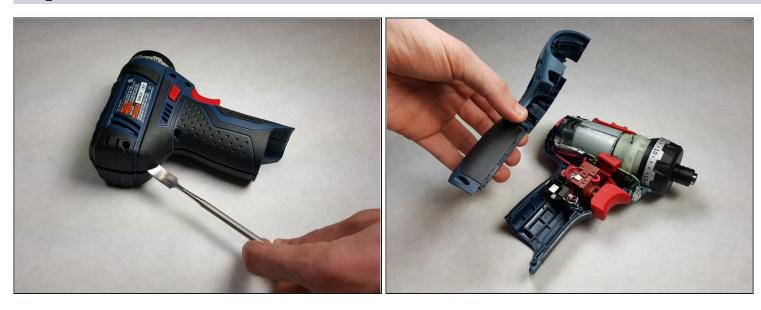
Remove the upper portion of the case from the outer portion of the case using a metal spudger.
