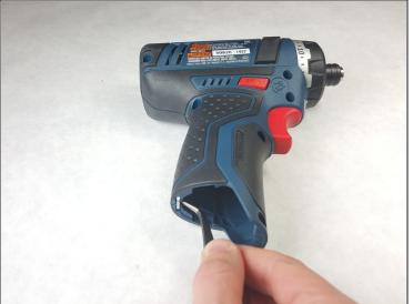
• Locate the clip that binds the two halves of the outer casing together on the rear edge of the battery shaft. Remove the clip with the angled <u>tweezers</u>.
