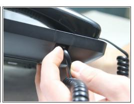
Locate the plug-in jack on the bottom right side of the phone.
