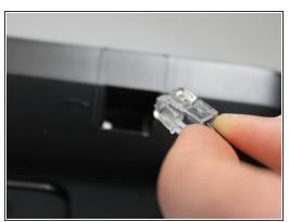
Pinch the clip on the plug and pull the cord from the base in order to release the cord.
