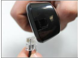
Pinch the clip on the plug and pull away from the handset in order to release the cord.
