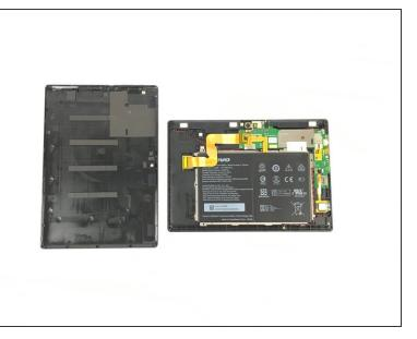
Use a plastic opening tool to pry open the back cover of the tablet.
