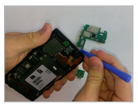
Use the plastic opening tool to pry the audio jack loose.
