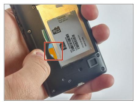
After the battery is removed, push the SIM card from the left side with your thumb until it is loose.
