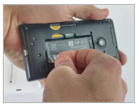
Once the cover has been removed, the battery will be visible. Grab the plastic tab and pull it to remove the battery from its place. If there is no plastic tab, use the plastic opening tool to pry the battery loose.
