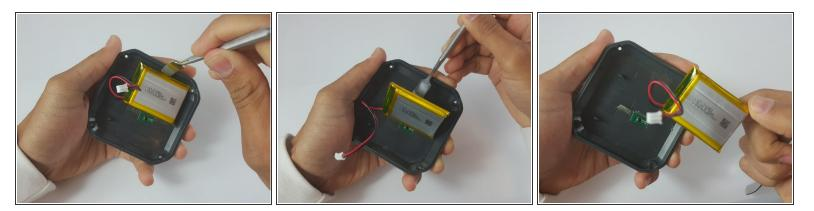
Use the metal spudger to carefully pry along the entire side of the battery from its connecting tape on the back cover.
