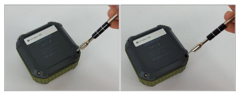
• Use a magnet to remove the screws after unscrewing them and place them aside.
