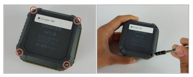
• Use a T6 Torx screwdriver to remove the four 9mm screws from the back of the device.
