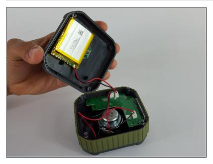
Carefully remove the back cover without breaking the battery wire.
