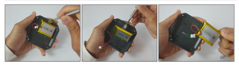
• Use the metal spudger to carefully pry along the entire side of the battery from its connecting tape on the back cover.
