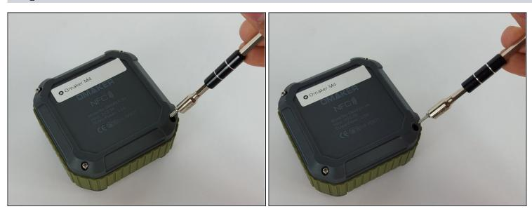
• Use a magnet to remove the screws after unscrewing them and place them aside.
