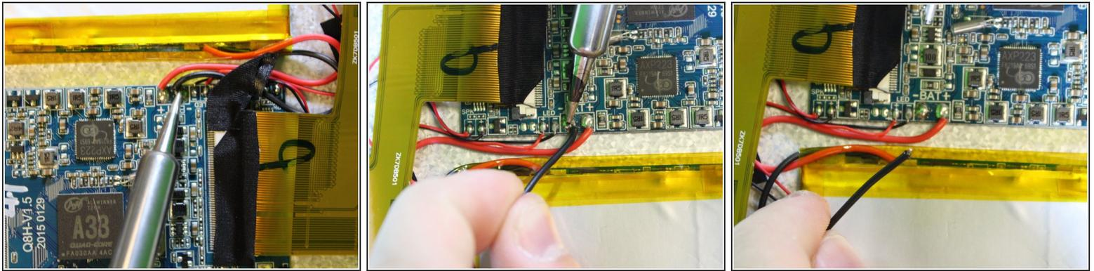
**⚠** The soldering iron can destroy components on the motherboard. Only touch the soldering iron to the solder already on the board.
