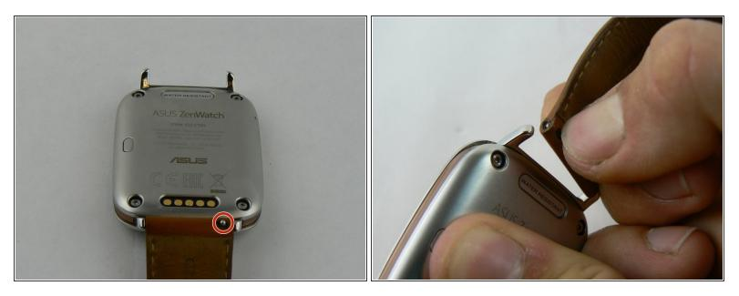
• On the strap there is a knob. Sliding this knob towards the opposite side of the strap releases the tension on the spring bar, allowing you to pull the strap out..
