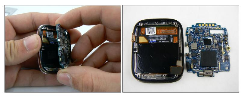
• With all the connections disconnected the motherboard can be gently pried up and out of the watch case.
