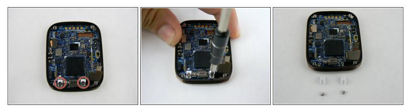
With the 000 Philips screwdriver remove the screw and plastic retainer clips
