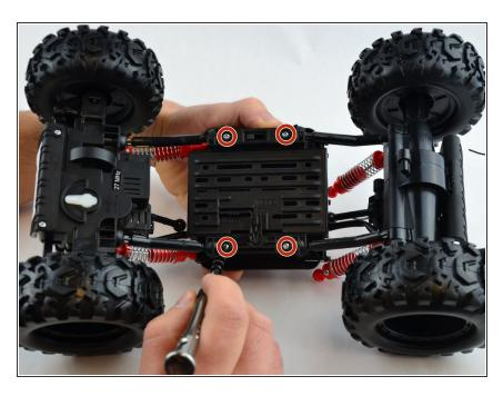
Flip the R/C truck over and remove the four 10 mm bottom under-body plate screws using the driver and bit PH2.
