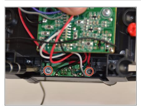
After removing the plate use the driver and bit J1 to unscrew the two 9.5 mm Phillips screws that hold the side circuit board in.
