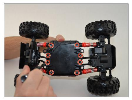
Use the Driver and bit J1 to remove the top under-body plate by unscrewing the eight 9.5 mm Phillips screws.
