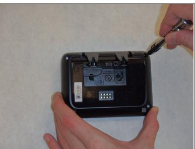
Remove the four Phillips #0 screws (9.4mm) located at the bottom of the phone on the back side of the base.
