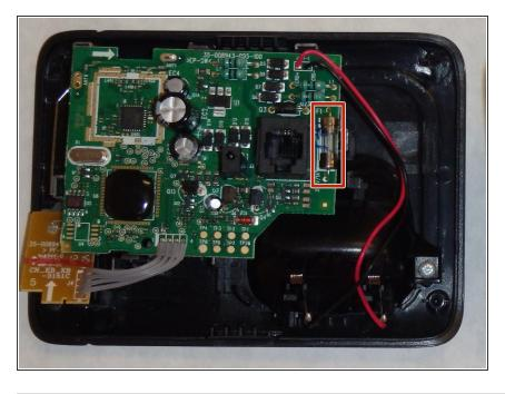
Flip the board back over and remove the fuse.
