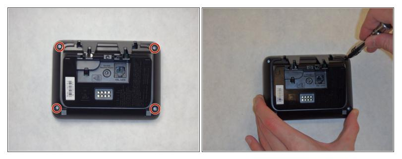
Remove the four Phillips #0 screws (9.4mm) located at the bottom of the phone on the back side of the base.
