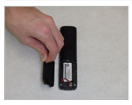
Pull the battery cover off of the back of the phone.
