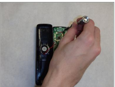
Remove the two 9mm screws located inside the back cover at the top.
