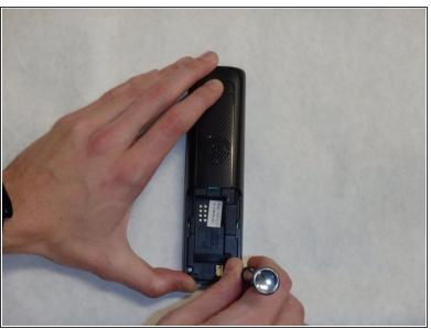
Remove the two 9mm screws on the back side with a Phillips #0 screwdriver.
