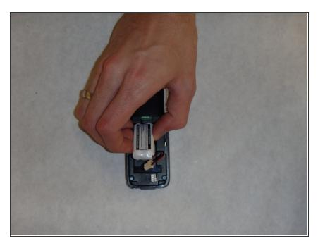
Lift the battery out of the back of the phone.
