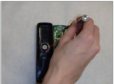
Remove the two 9mm screws located inside the back cover at the top.
