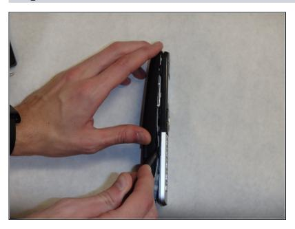
Use the plastic opening tool and spudger to pry the back side of the phone off.
