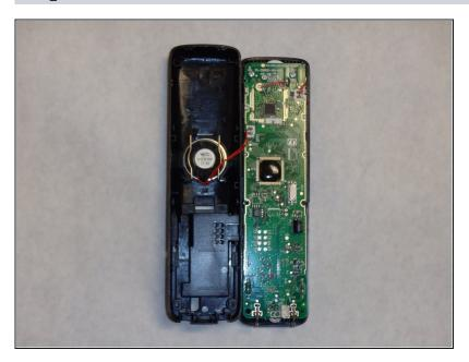
Heat up solder joint on the circuit board where the speaker wires are connected.
