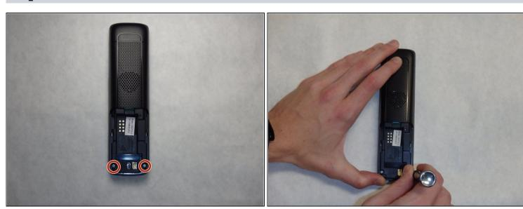
• Remove the two 9mm screws on the back side with a Phillips #0 screwdriver.
