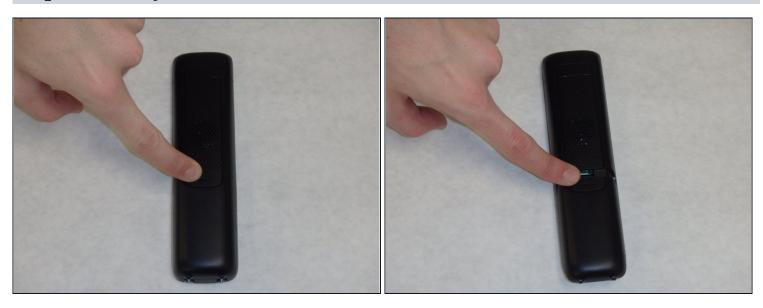
• Push down on the battery cover in the direction of the arrow located on the back of the phone.
