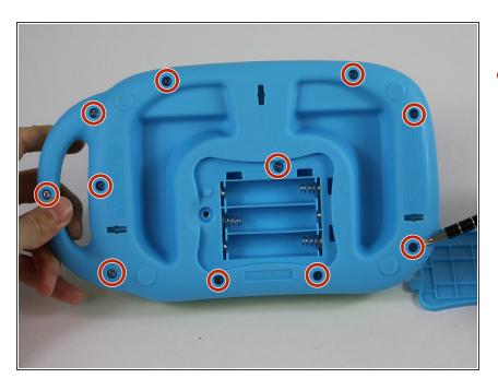
Remove the eleven 10mm screws from the back of the device with a a PH1 phillips head screwdriver.
