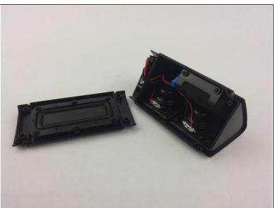
• Use the plastic opening tool on one of the corners to separate the bottom piece from the speaker, and then remove the piece.
