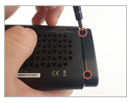
Remove four (4) 11.7 mm Phillips #0 screws from each side at the bottom of the speaker.
