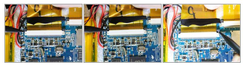
• Push both side buttons away from the socket by using a spudger.
