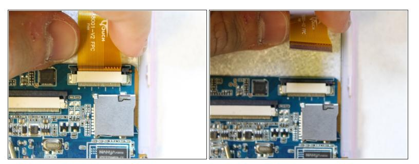
• Gently pull on the ribbon cable, separating it from the socket.
