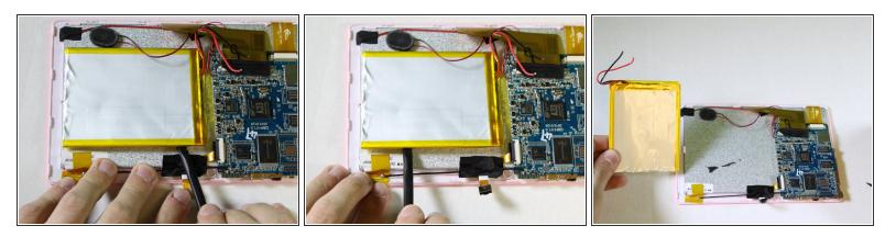
Use the nylon spudger to pry the battery from the back of the screen. Work your way around the edges, similar to opening the casing.
