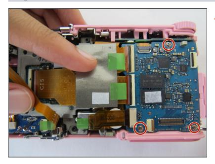
Move towards the main frame of the camera and locate the three 1mm Y0 screws holding down the motherboard.
