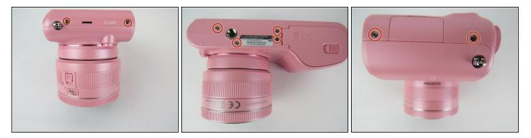
• Remove the 4mm Y0 screws found on the sides and bottom of the camera.
