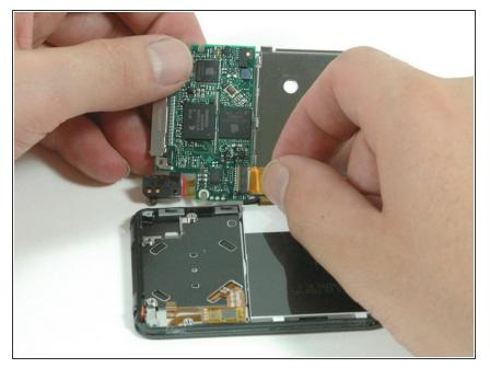
• We've disconnected the click wheel cable and flipped the board over to disconnect the display cable.
