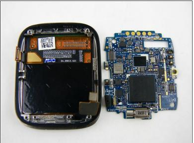
With all the connections disconnected the motherboard can be gently pried up and out of the watch case.
