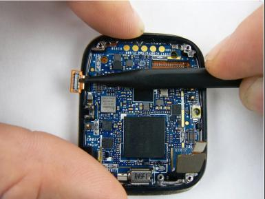
• With heavy duty spudger lift up on final connection ribbon located on left corner.
