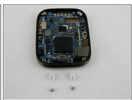
With the 000 Philips screwdriver remove the screw and plastic retainer clips
