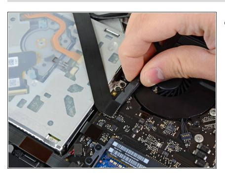
Use the flat end of a spudger to carefully pry the AirPort/Bluetooth ribbon cable up off its socket on the logic board.
