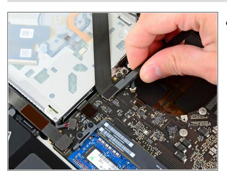
Use the flat end of a spudger to pry the AirPort/Bluetooth connector up from its socket on the logic board.
