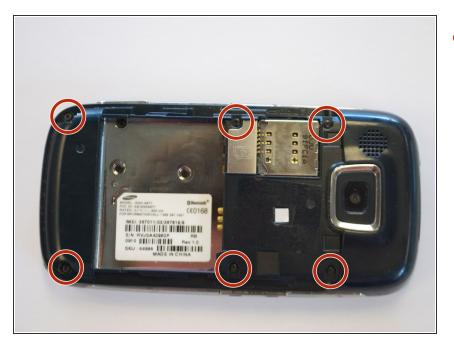
Remove the six 3.5 mm screws using a Phillips #000 screwdriver. Make sure to unscrew in a counterclockwise direction.
