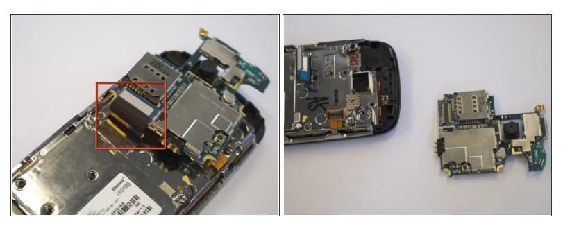
The circuit board will still be held on by a blue and black ribbon. Remove the entire circuit board by gently tugging the ribbon upwards.
