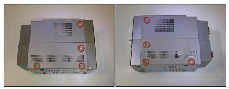
• With a Phillips #0 screwdriver, remove the eight 9.5mm screws attached to the left and right panels of the device.
