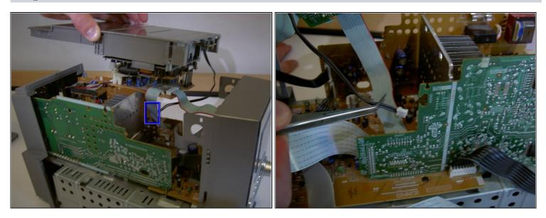
Disconnect the black wire by gripping the wire at the base and pulling gently until released.
