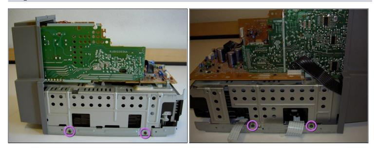
• Using a philips screwdriver, remove the four 9.5 mm screws indicated and place aside.
