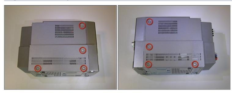
Using a Phillips screwdriver, remove the eight 9.5 mm screws on the left and right sides of the device.
