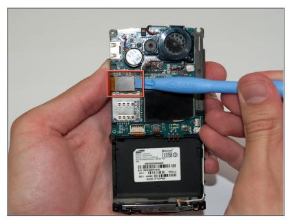
Using iPod opener tool, unlatch LCD ribbon cable on left side of motherboard.
