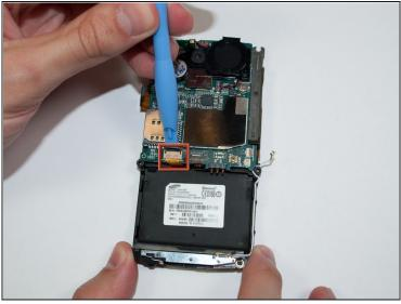
Using iPod opener tool, unlatch and remove the two ribbon cables at the bottom center of motherboard for the keypad and center button.
