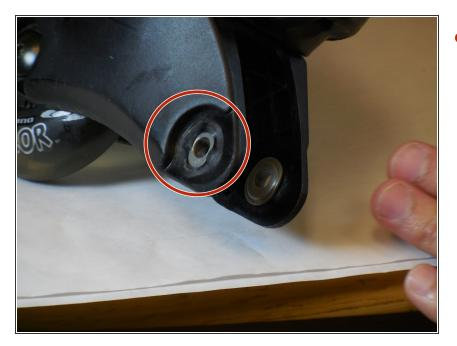
Retrieve the new plastic washer and insert between the blades on the inner side. Do the same to the other side, so that both sides have new plastic washers
