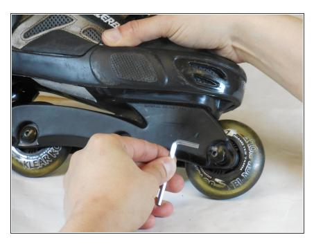
• Lastly, tighten the screws with the Allen Wrench.
