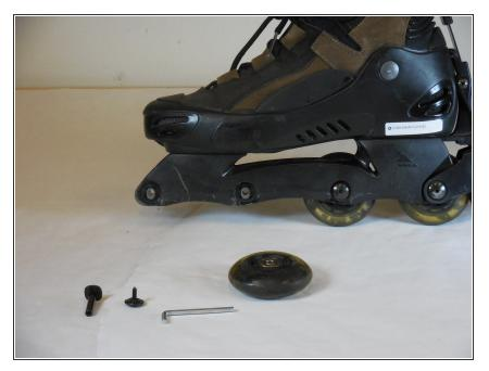
• Remove the screws and wheel from the blade.
