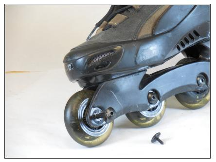
• Reinsert the screws through the plastic washers and wheel.
