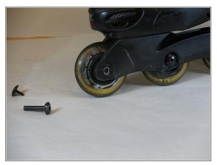
Replace the wheel without dislodging the new plastic washers and center the hole of the wheel in each plastic washer.
