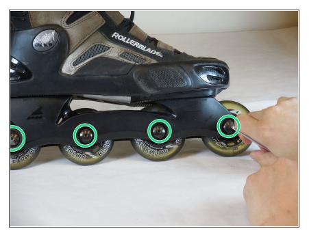
• Use an Allen Wrench to unscrew the screws on each side of the wheel.
