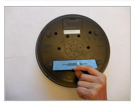
• Slide the battery cover off of the back.
