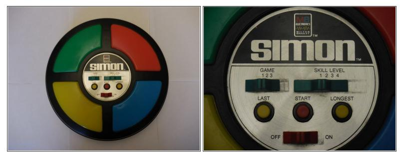
• Make sure the game is powered off by switching the On/Off switch to the left.
