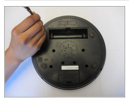
• Use the Phillips Head screwdriver to unscrew the screws located at the four corners of the game.
