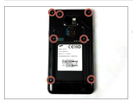
Use the Phillips screwdriver to remove the 7 Phillips head screws, indicated in the picture.
