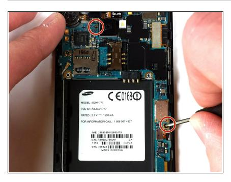
Remove the two black Phillips head screws located at the top left and the bottom right of the logic board.
