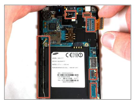
Disconnect all push connectors and the antenna cable with a small pull shown on the left.
