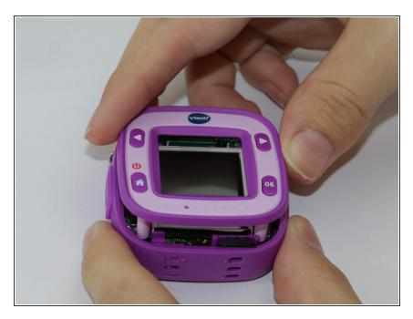
Turn the camera around and gently remove the plating that surrounds the LCD screen by grasping it with your fingers and pulling away from the device.
