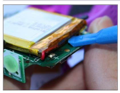
Gently lift the battery away from the motherboard using a plastic opening tool.
