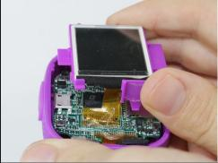
• Use the plastic opening tool to lift the LCD screen, including the purple casing and set it aside, revealing the motherboard and connector ribbon.
