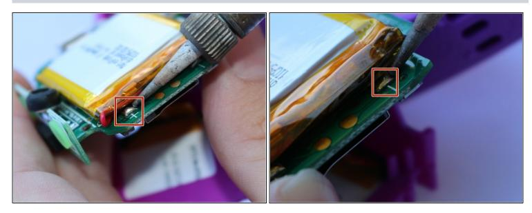
Use the soldering iron to unsolder the battery wires connected to the motherboard by reheating the existing solder.
