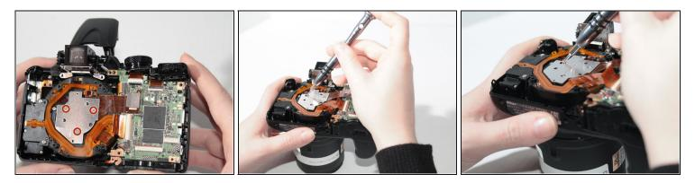
• Remove the 3mm screws highlighted in red using the Philips #000 screwdriver.
