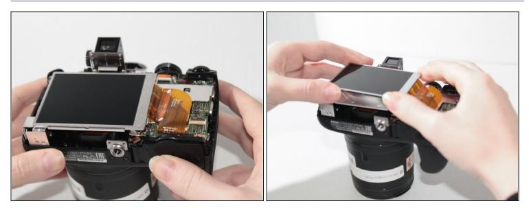
• Lift the LCD screen upwards.
