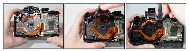
• Remove the four 7mm screws highlighted in red using the Philips #000 screwdriver.
