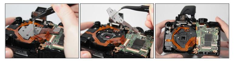
• Use the <u>tweezers</u> to remove the CCD sensor carefully.
