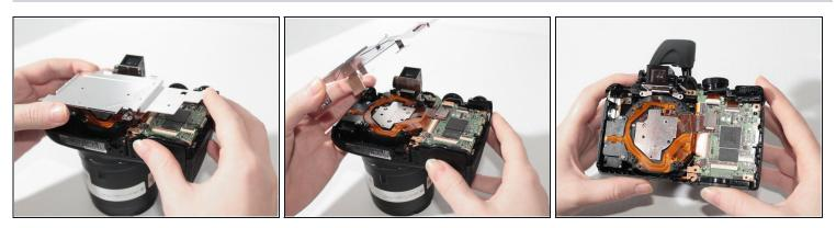
• Lift and remove the LCD mounting bracket to expose underlying hardware.
