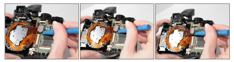
• Disconnect the ribbon cable connector by prying upwards on the part using the plastic opening tools.
