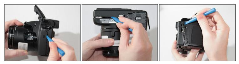
• Gently pry with a plastic opening tool around the perimeter of the camera.
