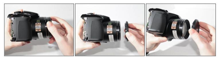
• Remove the lens cover to free the zoom motor unit from the camera body.
