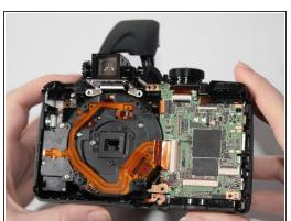
• Use the tweezers to remove the CCD sensor carefully.
