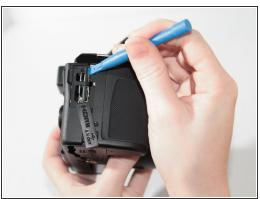
Gently pry with a plastic opening tool around the perimeter of the camera.
