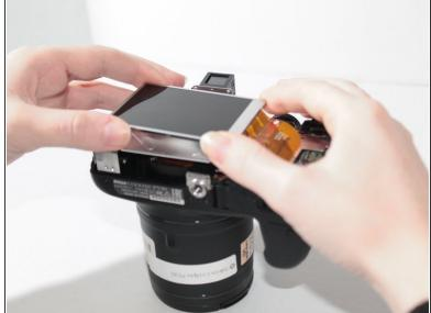
Lift the LCD screen upwards.
