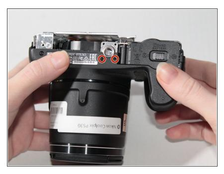
Identify two the remaining 4mm screws to be removed using the Philips #000 screwdriver.
