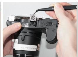
Once these screws have been removed, use tweezers to take out the tripod mount.
