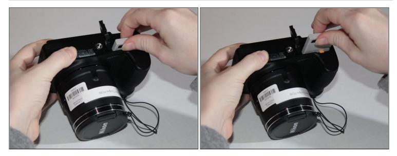
• Gently remove the battery from the chamber.
