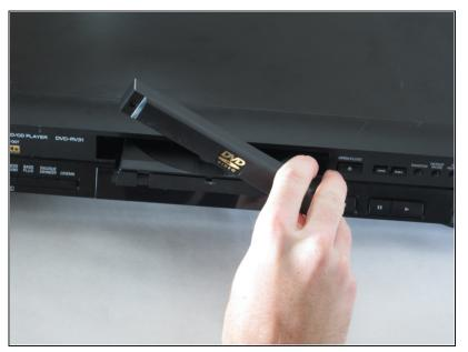
Evenly lift upward on the disk tray front cover (not slanted, as pictured). This will allow for easier disassembly of the player.
