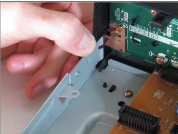
• Lift up the five tabs securing the front panel to the chassis. There are three on the bottom, and two on the inside edges of the panel. Panel should then lift off the player.
