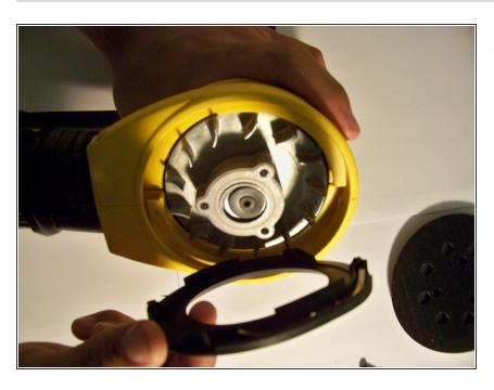
When the disc pad is removed, the brake is located directly under it.
