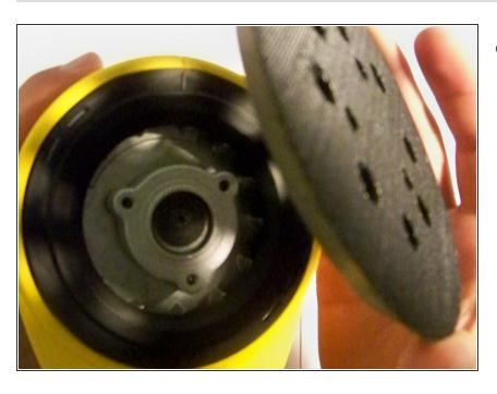
After the T20 torx bolts have been removed, remove the disc pad from the sander.
