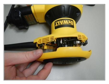
Once the cap is removed, the switch and connectors should be exposed
