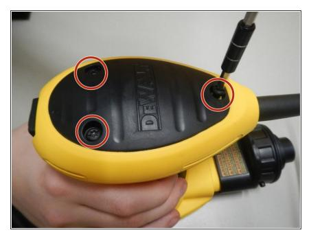
Remove screws (3) from the cap using a T20 torx attachment by unscrewing in a leftward motion
