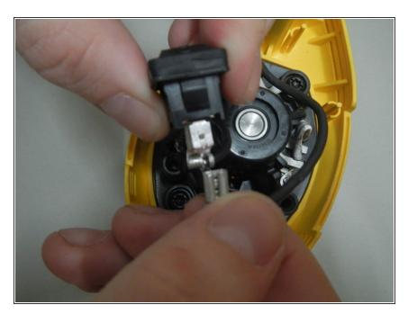
Remove both connectors from the switch
