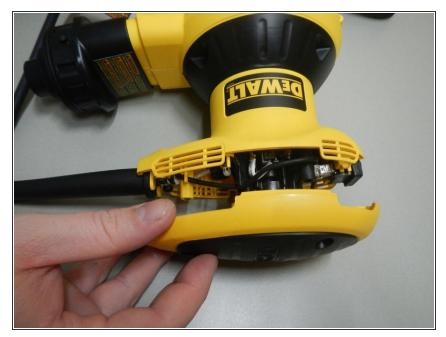
Once cap is off, expose and locate the power cord mounting bracket and remove the 2 screws holding the wire down by using the T15 torx attachment. Once the cord is loose, pull the connectors out
