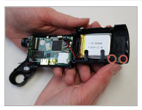
Locate the two screws that attach the tripod nut to the device.
