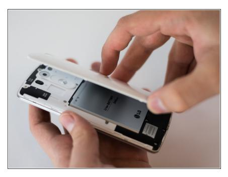
Gently pull the cover on the back of the phone off to locate the battery.
