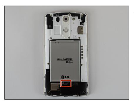
Remove the battery by lifting from the slot at the bottom of the battery.
