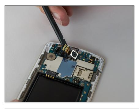
Use the spudger to gently unplug the ribbon cable connected to the motherboard. Then remove the rear facing camera.
