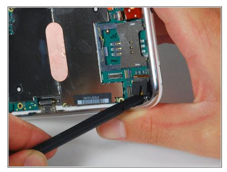
Use a spudger to gently pry the camera up and out of its housing in the rear panel. The camera cannot be removed entirely yet because it's connected to the bottom of the logic board.
