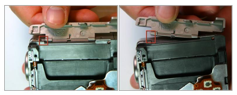
• Remove the CF card door from the left side of the camera body.
