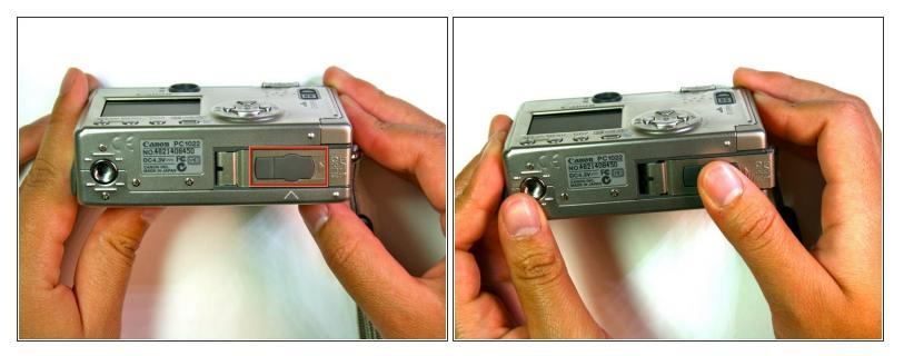
Slide the grey latch to open the battery compartment.
