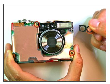
• Remove the two 3.9mm screws that hold the laminated copper sheet.
