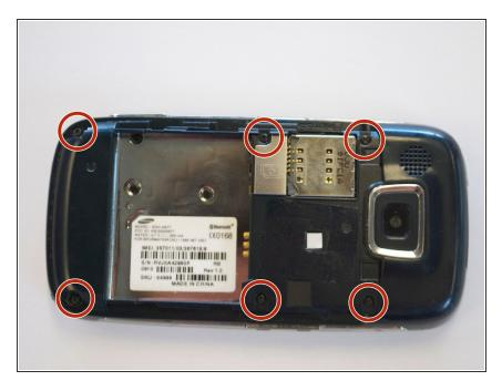
Remove the six 3.5 mm screws using a Phillips #000 screwdriver.
