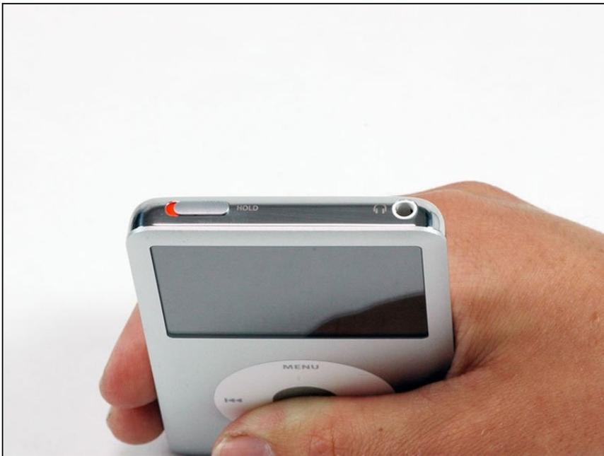
ⓘ Apple designed their new iPods to be very difficult to take apart without destroying major components. Because of the metal faceplate, the metal backing, and the 13 (yes, 13) metal clips holding the case together, this is one of the toughest iPods to disassemble.
