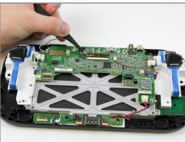
• Carefully lift the black clasp. It is prone to breaking if only lifted from one point. Remove the brown ribbon by using the tweezers.
