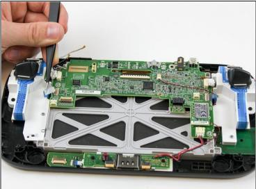
• Remove the blue connector using tweezers.
