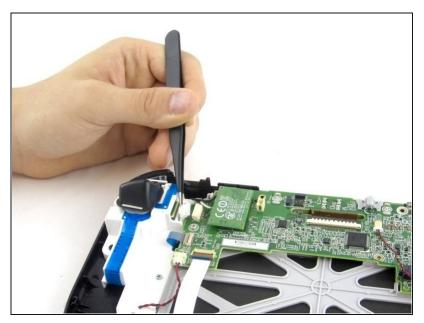
• Disconnect the analog connector with tweezers.
