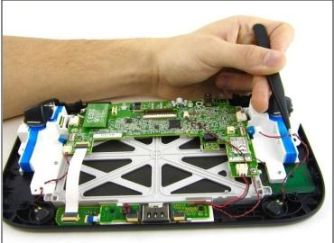
• Remove the right speaker cable that's connected to the motherboard with the tweezers.
