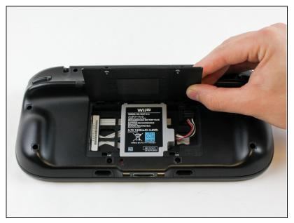
• Lift and remove the battery plate.
