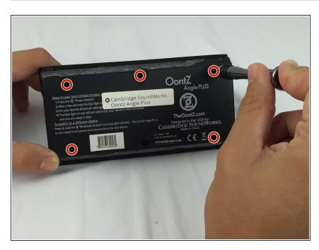
Unscrew the five 11.5mm Phillips screws from the bottom plate.
