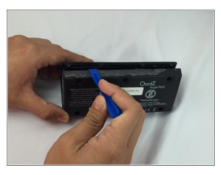
Carefully pull apart the bottom and top plates, using the blue plastic opening tool.
