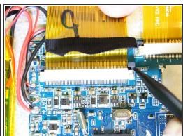
Push both side buttons away from the socket by using a spudger.
