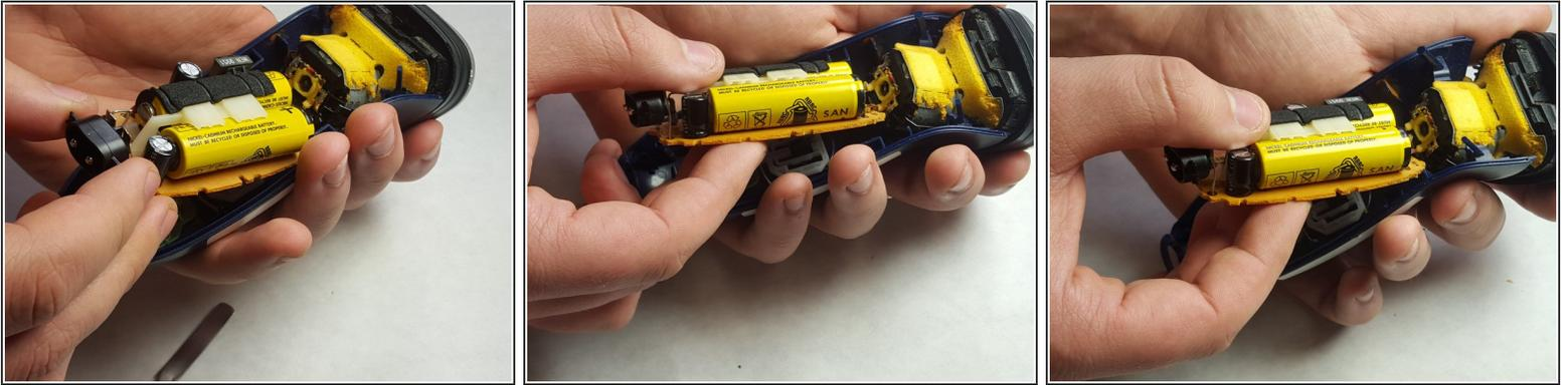
**⚠** Cautiously lift and twist the circuit board, then begin sliding the inside assembly forward.
